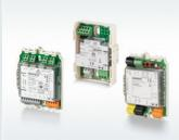
Input/output modules further increase safety and security. With the input modules FDCI221/FDCI222, you can monitor the status of doors, ventilation or sprinklers. The input/output modules FDCI0221/FDCI0222 enable decentralized control of fire doors and plant. The "transponder" FDCI0223 enables a monitored connection of conventional detector lines, alarm signaling devices and devices in explosion-protected zones.
